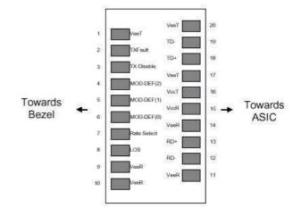
SFP Transceiver Electric Pad Layout
