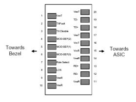
SFP Transceiver Electric Pad Layout
