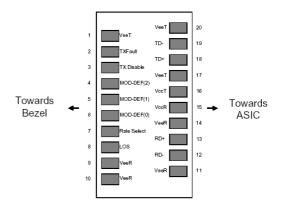
**SFP Transceiver Electric Pad Layout**
