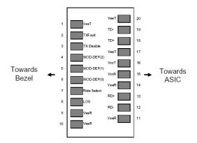
**SFP Transceiver Electric Pad Layout**
