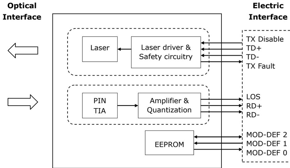
The transceiver is fundamentally consisted by two parts: transmitter and receiver. The transmitter features a TTL logic level Disable signal and a Fault indicator. The receiver features a TTL logic Loss of Signal (LOS) detection. For the access of serial identification information, an EEPROM is used to store the required data via the 2-wire serial CMOS EEPROM protocol. The detailed signal descriptions are listed in the following sections.
